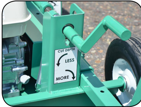
Depth adjuster in work position Press down on handlebar for travel mode
