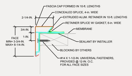
PRE-DRILL WITH 3/16-IN. DRILL BIT FOR MASONRY CONDITIONS.
